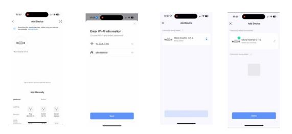
Connect PV cable to micro inverter, then press RESET (WiFi button) and hold for 3 to 5 seconds, click **Add Device** from up-right of the Smart Home App, you will see device(s) listed, click one of the devices, and enter your Wi-Fi password, **make sure the frequency of WiFi is 2.4GHz**. Then click **Next** to add device, after it's done, click Done to enter the device control panel.
