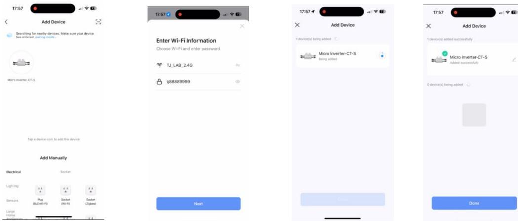
Connect PV cable to micro inverter, then press RESET (WiFi button) and hold for 3 to 5 seconds, click **Add Device** from up-right of the Smart Home App, you will see device(s) listed, click one of the devices, and enter your Wi-Fi password, **make sure the frequency of WiFi is 2.4GHz**. Then click **Next** to add device, after it's done, click Done to enter the device control panel.
